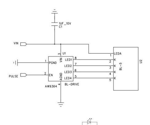
Note: constant current circuit for every LED, and though LED lamp current is less than 20mA. Recommand between 15mA and 20 mA for every LED.
